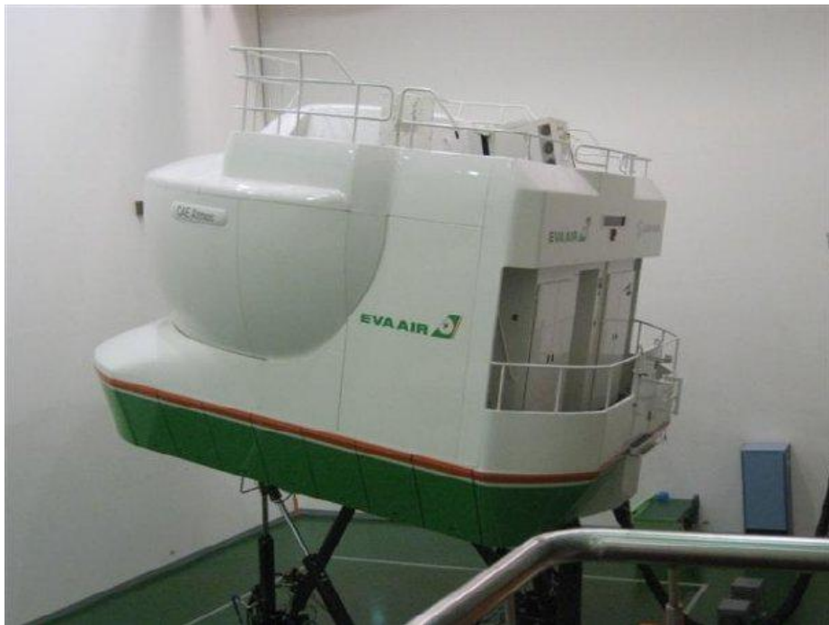
Realistic flight simulator used to train EVA Air pilots
